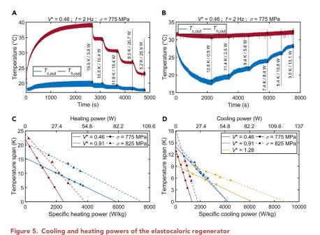
(A and B) Time evolution of the temperature span due to the gradual increase of (A) the heating power in the heat-pumping mode and (B) the cooling power in the cooling mode.
