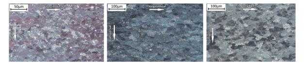
Fig. B.16. Grains of the tubes: Dt25 at 200× magnification (left), Dt12 at 100× magnification (middle) and Dt5 at 100× magnification (right).
