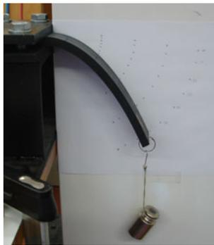
Fig. 7 Measurement of deflections of the beam
