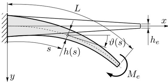
Fig. 2 Pure bending of non-prismatic cantilever beam
