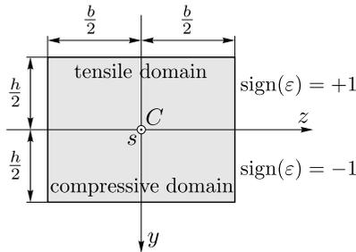
Fig. 3 Cross-section of the cantilever beam
