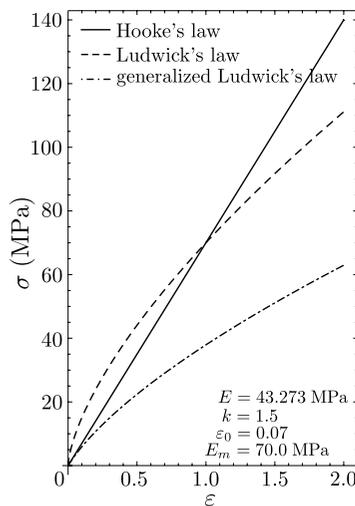
**Fig. 5** Stress–strain curves for Hooke, Ludwick and generalized Ludwick type elastic material
