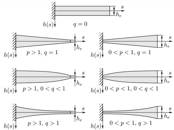
Fig. 4 Longitudinal shapes of the beam defined by (4)
