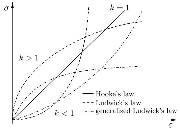
**Fig. 1** Stress–strain relations in tensile domain
