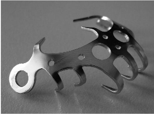
Fig. 7. Modified patellar basket plate before mechanical testing.
