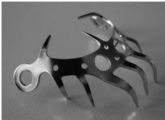
Fig. 9. Modified patellar basket plate after the mechanical testing.
