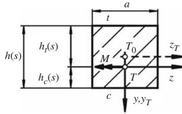
Figure 4. Rectangular cross-section of the beam.
