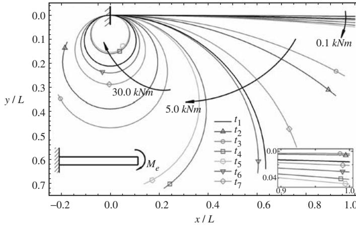
Figure 5. Deflections of the beams for Example 1.
