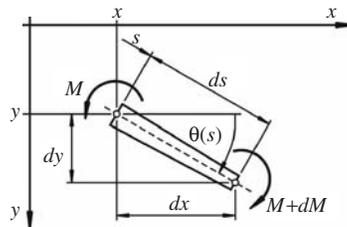
Figure 3. Infinitesimal element of the deflected beam.
