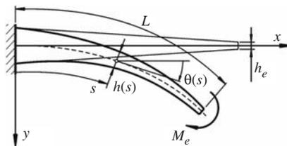
Figure 1. Bending of non-prismatic cantilever beam.
