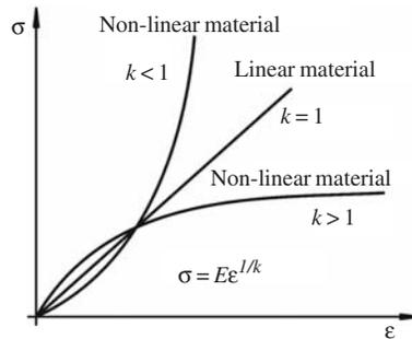
Figure 2. Stress–strain relation for Ludwick type material in tensile domain.
