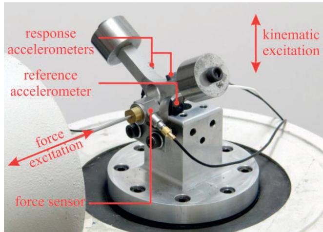
Fig. 1. Experiment setup.
