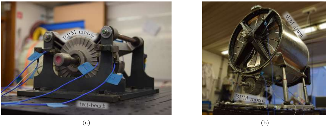
Figure 20: Experimental setup; a) a BPM motor on a test-bench, b) washing machine (WM) drum assembly.
