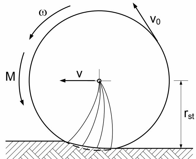
$$\begin{aligned} \frac{M_1}{r_{st1}} + \frac{M_2}{r_{st2}} &= F_{K1} + F_{K2} = \\ &= \left[ \frac{G}{g} + \frac{J_1}{r_{st1} \cdot r_{d1}} + \frac{J_2}{r_{st2} \cdot r_{d2}} \right] \cdot \ddot{x} + G \cdot \sin \alpha + R_z + \underbrace{R_{f1} + R_{f2}}_{R_f} + (R_p) \end{aligned}$$
