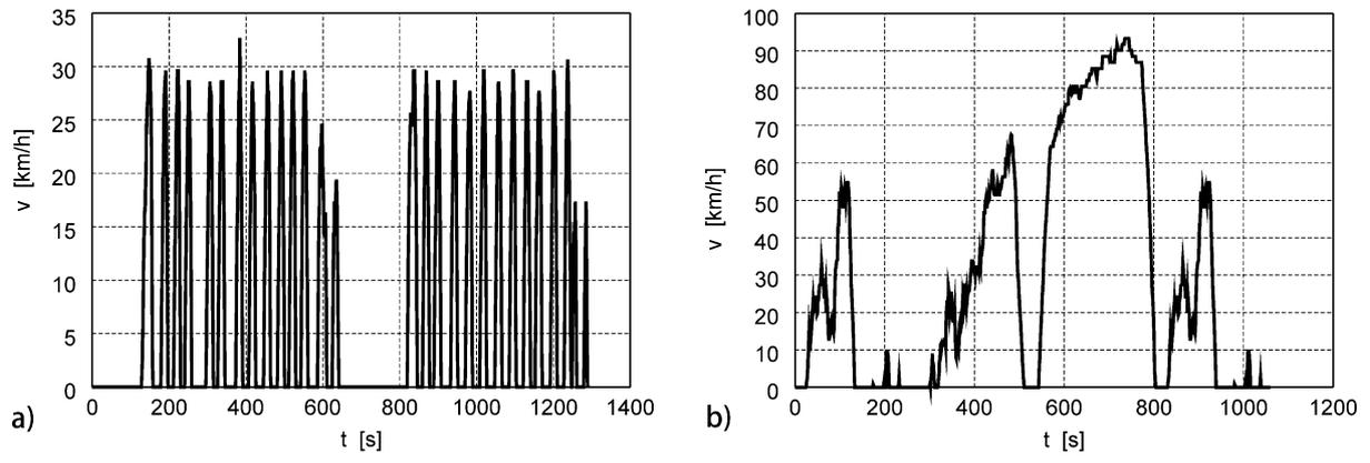
**Fig. 2** Velocity profile of: (a) BUSRTE, and (b) UDDSHDV drive cycles
