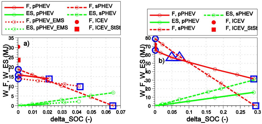
**Fig. 6** Energy depleted from the fuel tank ( $\Delta W_F$ ) and energy depleted from the batteries ( $\Delta W_{ES}^*$ ) of different powertrain topologies driven according to the (a) BUSRTE and (b) UDDSHDV drive cycle
