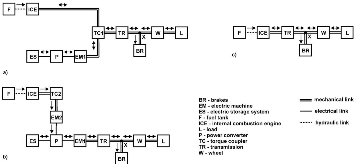
**Fig. 1** (a) Parallel and (b) series PHEV topology, and c) ICEV topology with indicated energy paths. Energy is added to the ICEV and parallel and series HEV only by the fuel (F), whereas parallel and series PHEV are also charged from an electric grid (ES).
