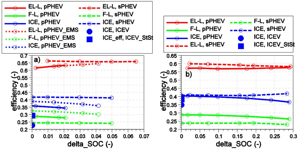
**Fig. 5** Energy conversion efficiency of the path from F to L ( $\eta_{F-L}$ ), energy conversion efficiency of the path from ES to L ( $\eta_{ES-L}$ ) and effective efficiency of the ICE ( $\eta_{ICE}$ ) of different powertrain topologies driven according to the (a) BUSRTE and (b) UDDSHDV drive cycle
