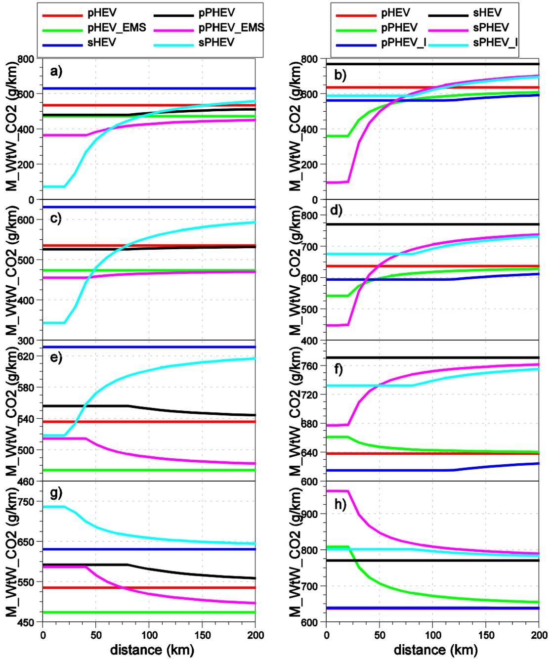
**Fig. 7** WtW CO<sub>2</sub> emissions ( $M_{wtW.CO_2}$ ) for the case of France – (a) BUSRTE and (b) UDDS HDV drive cycle; for the case of Europe – (c) BUSRTE and (d) UDDS HDV drive cycle; for the case of USA – (e) BUSRTE and (f) UDDS HDV drive cycle; and for the case of China – (g) BUSRTE and (h) UDDS HDV drive cycle. To preserve space in axis notation (g/km) is used to represent (gCO<sub>2</sub>eq/km).
