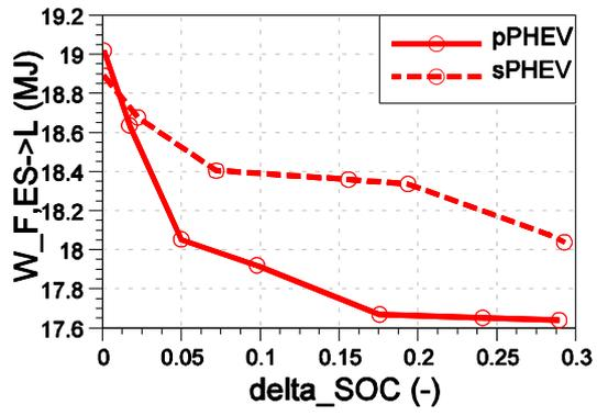
**Fig. 4**  $W_{F,ES \rightarrow L}$  of pPHEV and sPHEV driven according to the UDDSHDV drive cycle for different depletion rates of the electric storage devices
