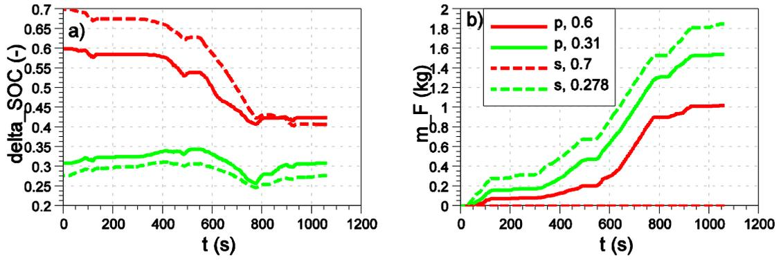
**Fig. 3** (a)  $\Delta SOC$  and (b) mass of the fuel consumed over the drive cycle ( $m_{F,dc}$ ) of the pPHEV and sPHEV driven according to the UDDSHDV drive cycle for different initial values of the SOC
